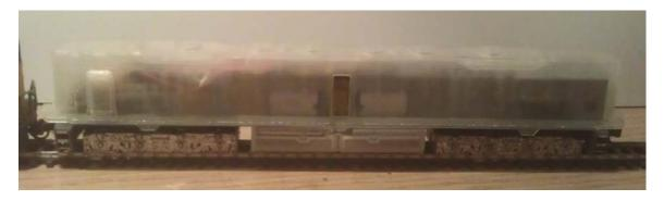
If you are feeling BRAVE, you can cut out the passageway through the chassis as in the photos on the next page. This was done before the four chassis parts were re-assembled. Using the body as a guide, cut down as far as the running board 3.5mm from each side. The plastic "spine" will now be in two parts, one at the top, one at the bottom, and two small "jumpers" were glued in the gap at the top (see 2<sup>nd</sup> photo).
