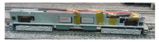
The shell should slip over the chassis and clip into place. The new fuel tank should also shape on in the same way.
