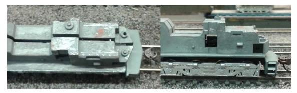
If you want to keep this as a DCC locomotive you will also need to remove the up stand in the cab area to make room for the chip as shown above right. When finished the cab area should look like this
