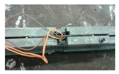
Using a strong glue, fix the 'H' shape to only one side, as you may need to disassemble the chassis for maintenance. If the chassis is for DC only, the two brown wires need to be attached to the right hand side of the chassis, the orange to the left. Also jumper wires need to run from the front to the back halves. Remember those screws? One hole needs to be drilled somewhere on the rear right chassis part and another screw found for that.
