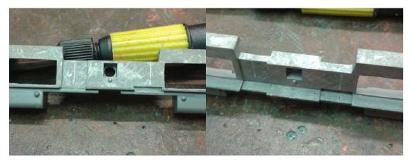
Once you have marked both side and <u>checked</u> that it is correct cut the centre part of each frame out with a hacksaw. You can cut them both at the same time if the end bolts are used minus the black plastic isolating washer to hold the halves together.
